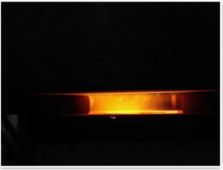
Design of a low emission fire wood continuous stove with new ideas -Ejector induced air flow and horizontal gasifier (EIGAS stove). The power drawn is 1.2 W for 4.5 kW thermal output. Eff. ~ 40 to 50 %
